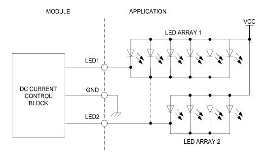
Figure 5.15-1 Typical circuit for LEDs
